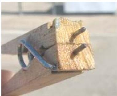
Cut the ends off a wooden clothes peg. Drill holes & insert piano wire.
