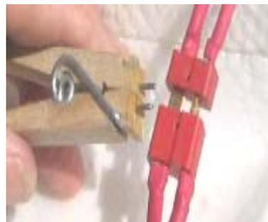
Drill a hole in the side of each Deans plug, a hair bigger than the piano wire and matching the distance between the pegs.
