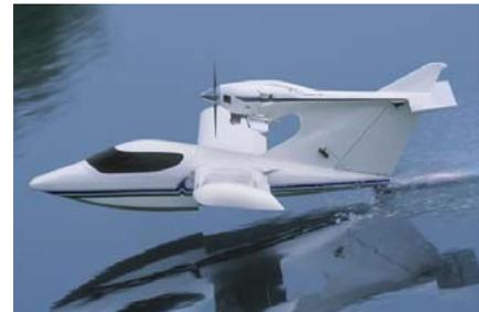
Both planes have similar engine mounting configuration and wing tip that double as floats. However, Great Planes *Seawind* has fixed landing gear with an option for retracts. Nitro Models *Seawind* has no provision for any landing, and claims that it can take-off from grass, skidding on its main hull. Note difference in Wing area.
