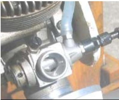
A good idle adjustment (a small "finger-nail" opening) should allow continuous idle for 5 minutes or more
