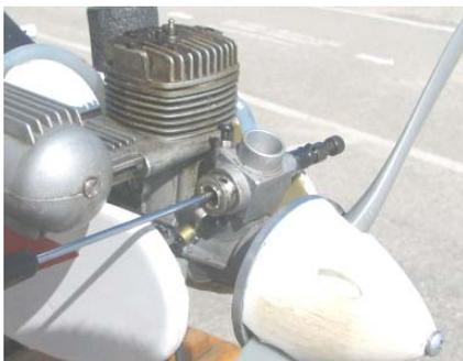
**Adjust the idle screw and listen for the change in rpm.**
