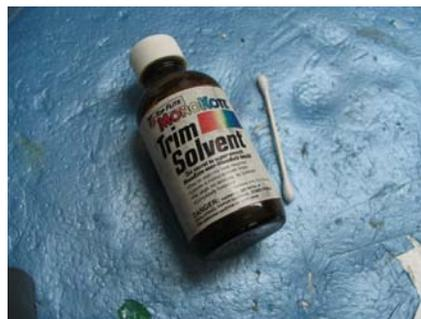
When you've finished covering your plane, or after a repair job, use a Q-tip dipped in Monocote solvent and run along all the seams. It will seep under the joint and make a seal that won't lift off.
