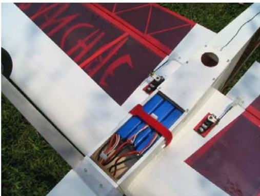
*The batteries are Velcroed to the plane, but I added the extra strap for double safety. The strap has an "eye" on one end, so it can be pulled tight then fastened*
