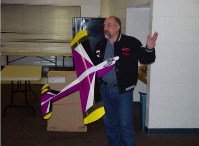
George Manning built this **Ringmaster** after it was shelved for 15 years! George uses the Ringmaster as an equipment test plane. Its fuselage is built up with balsa and aircraft ply, the covering is Monokote, Ultra Coat, and Solarfilm. Engine: Magnum .39; WS-57.5"; L: 37"; Fuel Tank: Dubro 8oz; Flight Time: 14 min.
