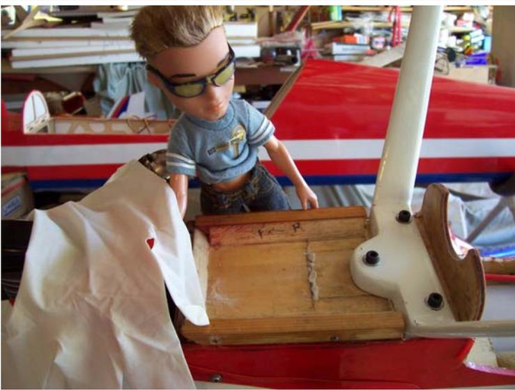
Here I am inspecting my Gorilla Glue repair job on my landing gear support area. Note how the glue expanded to fill the gaps. I have just taken off my latex gloves, which are necessary when using this product. By the way, it is moisture that sets up this glue. Read the directions carefully before using!
